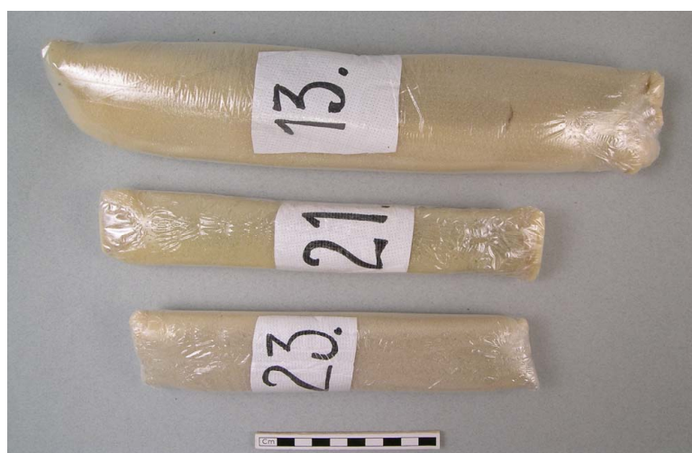
Plate 13. Artefacts supported by polyether foam and polyolefin film. (Copyright: National Heritage Board, Sweden).
