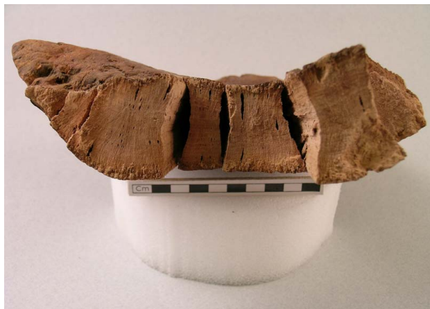
Plate 5. Example of salt precipitation and cracking. Detail of oar handle from Jukkasjärvi in Lappland, dated to Scandinavian Bronze Age (1800-500 B.C.). The specific treatment is unknown, but the presence of alum has been shown in SEM-analysis. (Copyright: National Heritage Board, Stockholm).
