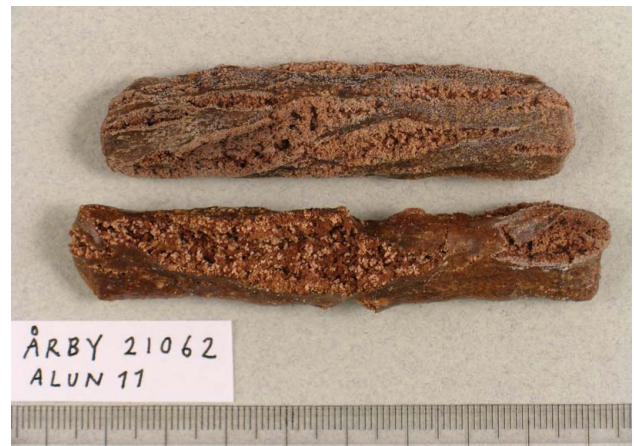
Plate 6. Example of surface flaking. Surface detail of a plank from Bulverket on Gotland, dated to Scandinavian Iron Age (500 B.C.-1050 A.D.). The specific treatment is unknown, but the presence of alum has been shown in SEM-analysis, and archival material strongly suggests glycerol has been added in the treatment. see 17-18. (Copyright: National Heritage Board, Stockholm).
