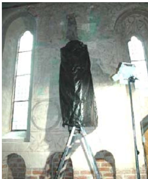
Figure 48. The “dark chamber” constructed for testing if the casein has been reduced in UV-light. Photograph Lena Östlund.
