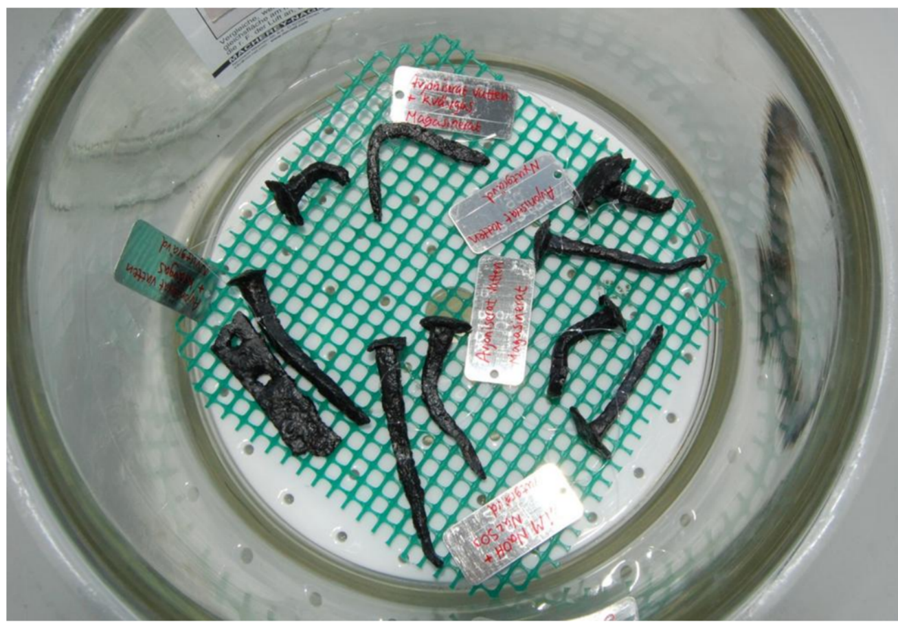
Test material in humidity chamber for corrosion test
