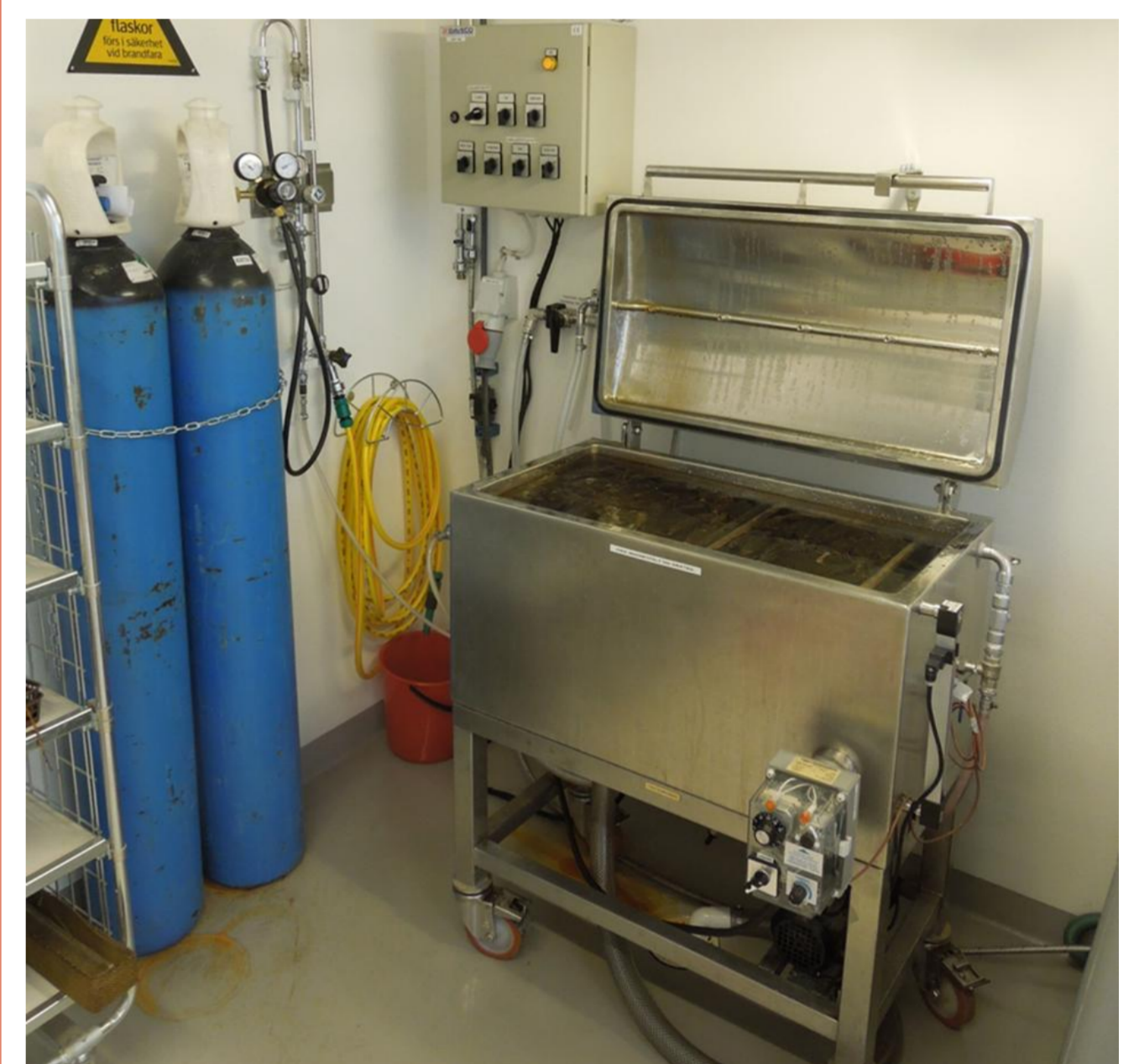
Desalination tank with Nitrogen flush system
