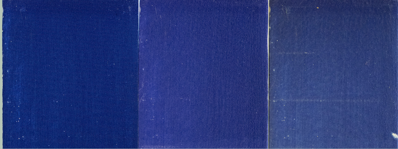
Smalt blue + egg-white mock-up. Left: before consolidation; Center: after consolidation with JunFunori 1%; Right: artificially aged.
