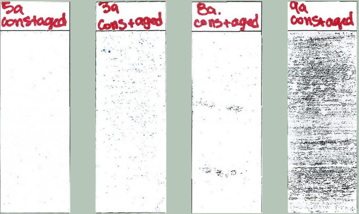
Tape tests of the artificially aged consolidated mock-ups (from left to right): 5a: sturgeon glue 3%; 3a: Lascaux's MfC 25%; 8a: Lascaux's MfC 100%; 9a: Lascaux's MfC 25%.
