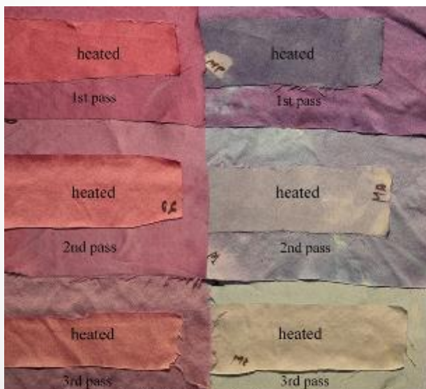
Silk dyed with 6-bromoindigo (right column) and 6,6'-dibromoindigo (left column)
